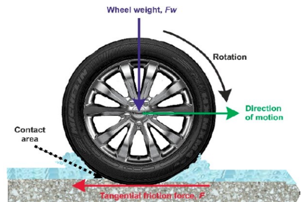
Figure 3. Various forces in action during a tyre-pavement interaction [33].
