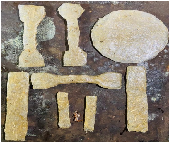
Figure 4. Weight percent fraction of the hybrid composite samples before precision machining.
