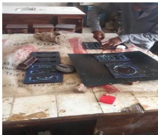
Figure 3. Open mold hand lay-up technique.
