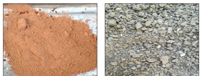
Figure 2. Brick waste and Road demolition wastes.
