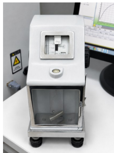
Figure 4. The analytical balance used in equilibrium swelling measurements.
