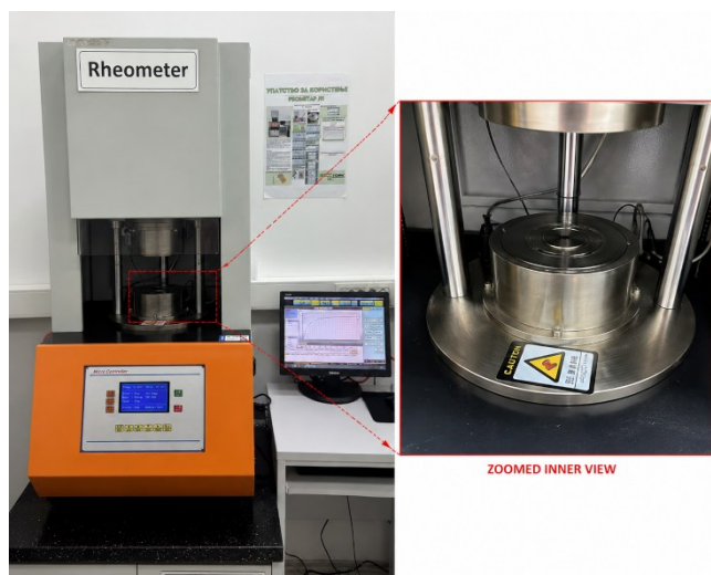
Figure 2. Moving die rheometer used for rheometric characterization of the investigated rubber compounds.
