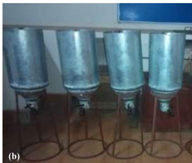
Figure 3. (a) Schematic view of the lime leaching test setup; (b) Experimental tanks used for lime leaching studies in the laboratory.
