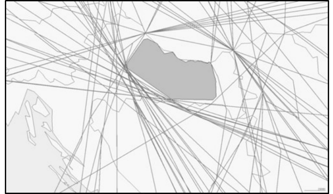
Figure 2. Civil air traffic trajectories in the case of LDTR24-27 activated at FL325-FL660.
